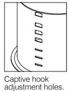
11. Lock the captive hooks and make sure the hooks apply a pressure against the ceiling to maintain the can firmly in place.
