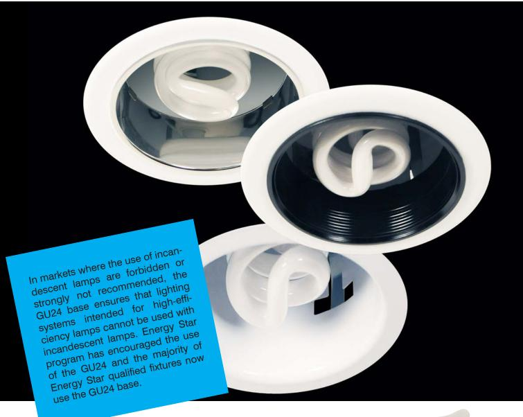
The GU24 base fixture has two receiving holes instead of the threaded receiving socket we are used to seeing on the Edison fixture. GU24 lamps are equipped with a pair of pins to match the fixture, and installation requires a simple insertion and twist to lock the lamp in place. These lamps are shorter, no need for the threading used in Edison fixtures and incandescent lamps are not available with the GU24 base.
